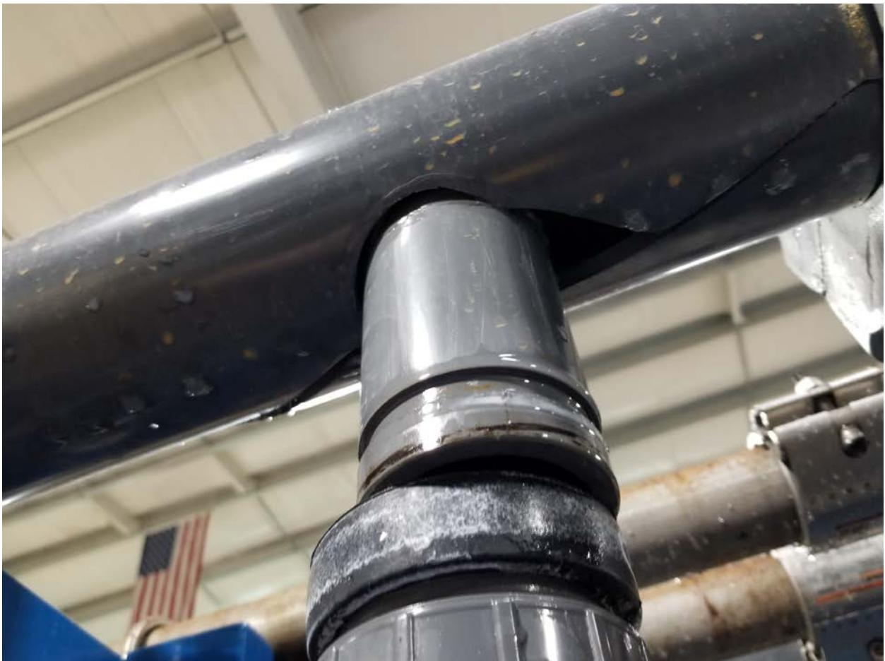
It also caused a filter cartridge to push up into the manifold, damaging it.
