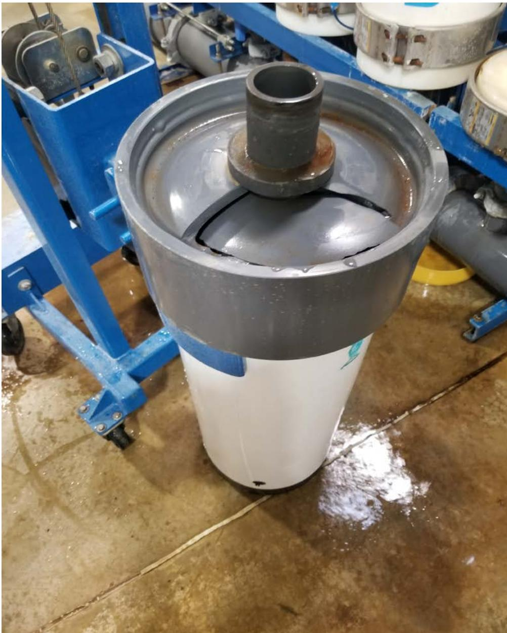
This pressure surge caused this filter cartridge to burst
