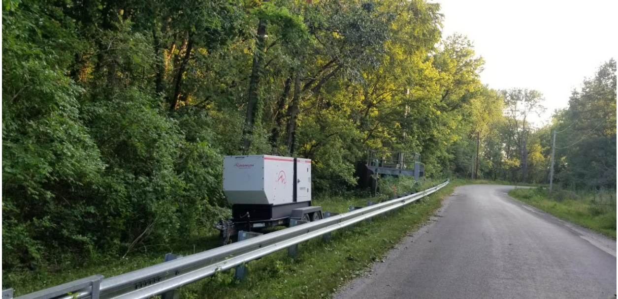
When the storms came through the booster station lost power. Lee electric brought a generator out to provide power. The generator had to be started and monitored numerous times a day.
