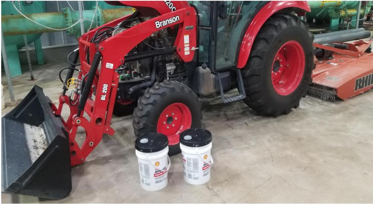
A full service was performed on our tractor which includes all oils and hydraulic fluids.
