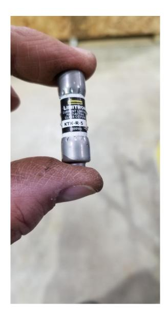
The actuator in the air valve being seized caused the fuse to weaken. Once it was freed the increased amp draw caused the fuse to blow. Once replaced the control valves began operating as they should.
