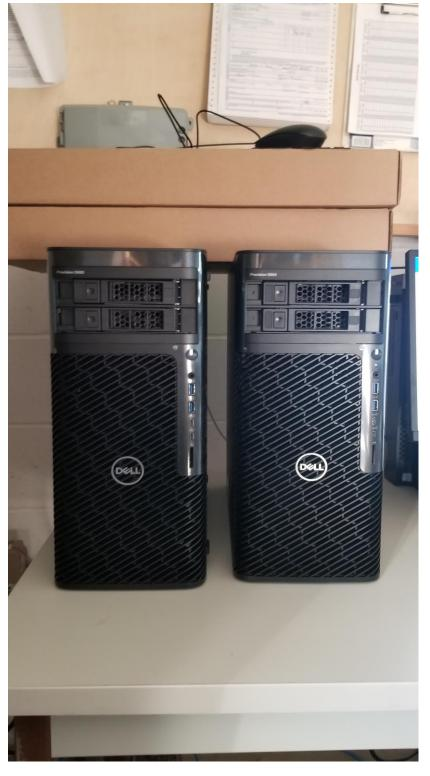
The scada computers that arrived onsite were unpackaged and power was put to them to ensure operation. Once powered up the computers were attached to the plant network. This will allow SCADAware to program the computers remotely.
