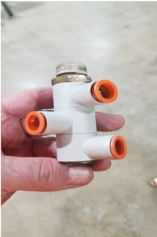
The air scour on train #1 came apart and had to be repaired.
